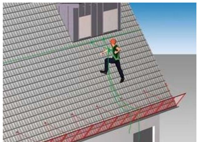
14 Rope access. As an additional measure, a roof safety barrier has been installed to catch falling material.
