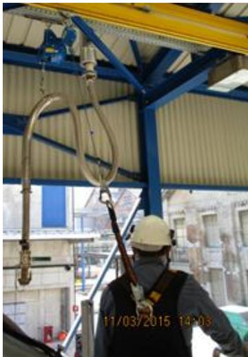
Fig. 11: Safety harness with fall arrester
