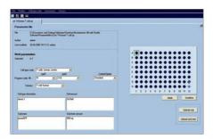
c) Result files (\*.ur): A result file is generated out of a parameter file as soon as the user starts a 96-well Nucleofection™ Experiment. The result file inherits all information of the parameter file and additionally logs the results of the Nucleofection™ Process.
